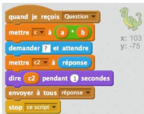
Scratch script for Exercise 4 continuation. It is triggered by 'when I receive Question', sets 'c' to  $a * b$ , asks '?' and waits, sets 'c2' to 'réponse', says 'c2' for 1 second, sends 'réponse' to all, and stops the script.
